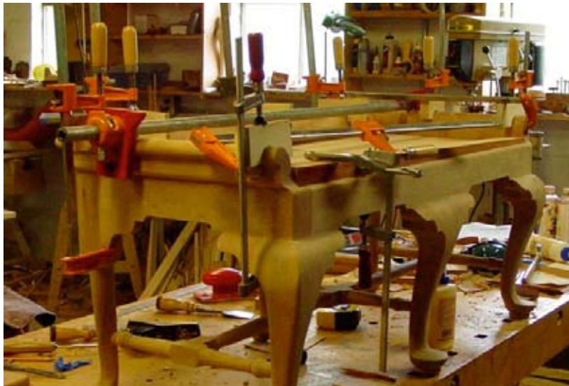
Although not the frenzied glue-up described in this story, this picture of a Queen Anne love seat depicts a successful but very uncooperative assembly! When you use clamps to clamp clamps so that your clamps will not . . . oh, well, you get the idea.
