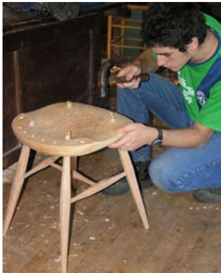
Scott's son Holden hammering a wedge into the tapered through-tenon of a Windsor chair seat (above)
