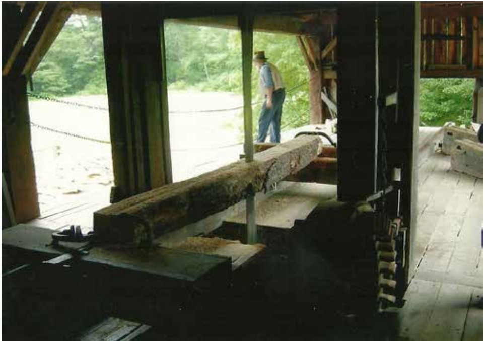
Operating water-powered up-and-down sawmill at Old Sturbridge Village where Bell made handmade reproductions of period furniture. The sawmill is a reproduction of the 19th century Nichols-Colby Sawmill of Bow, New Hampshire.
