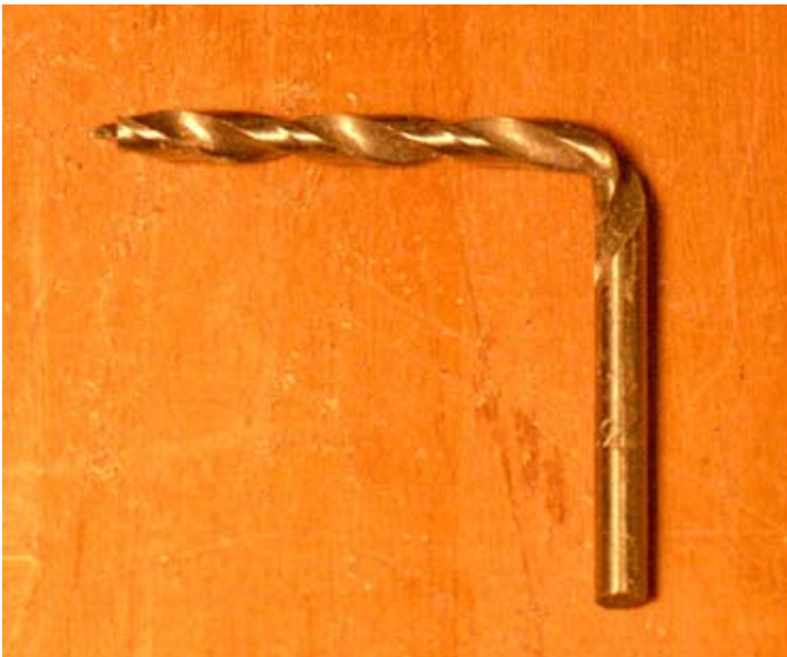
Special, more flexible steel must be used in this new type of right angle bit.
