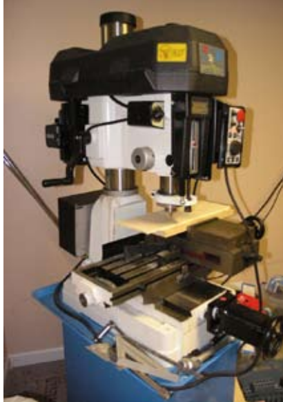
The "Mill Drill" is a small scale CNC
