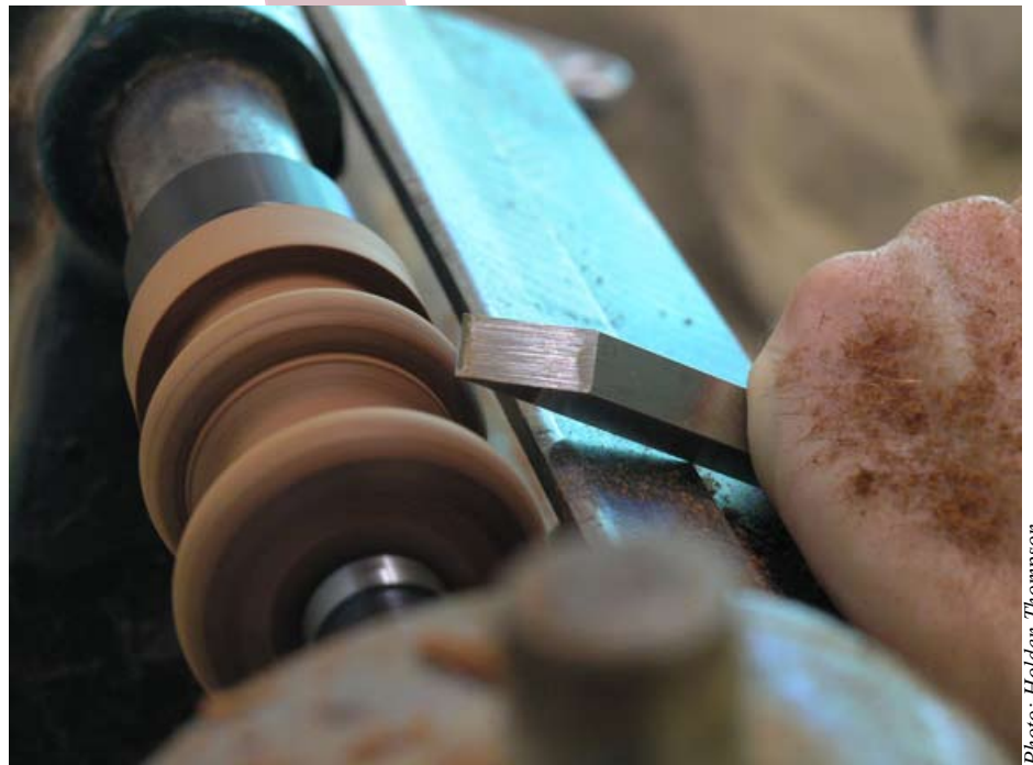
The bedan working at what it does best—shaping beads and round-overs.
